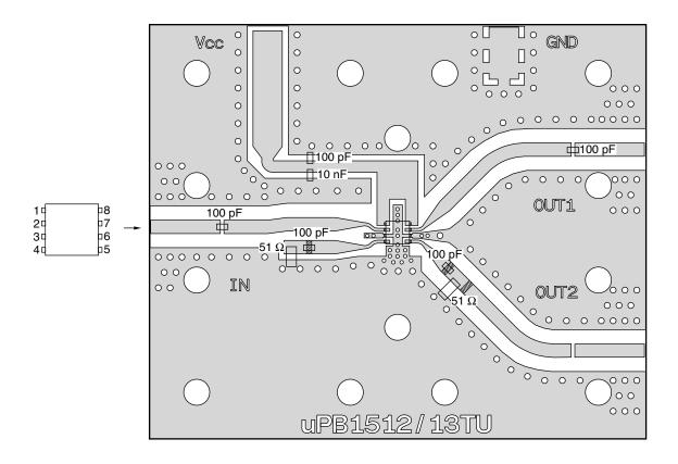
**Remarks 1.**  $33 \times 21 \times 0.4$  mm double-sided copper-clad polyimide PCB
